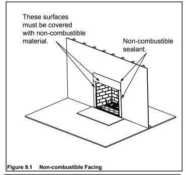
Note: We recommend mortar be applied after facing materials are installed. Refer to Section 7.E
